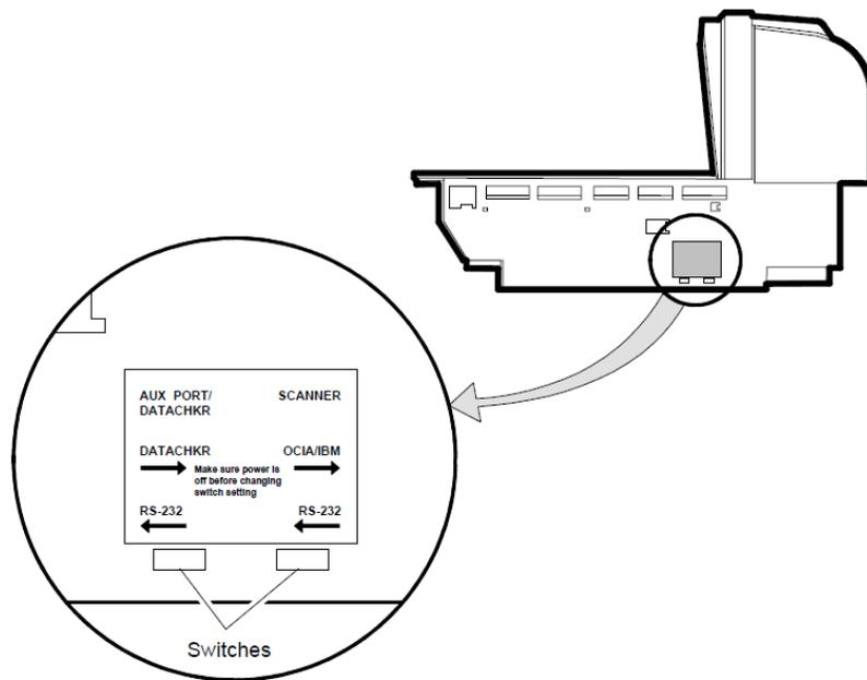
4. On the side of the scale make sure that the switch or switches are set to the RS-232 position.
