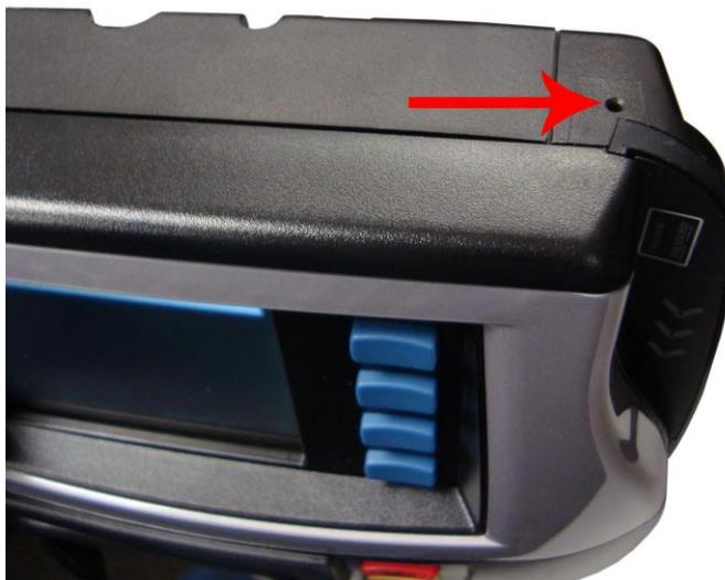
2. Using a narrow tool such as a paperclip press the button in the hole to reset the device, it may take a minute or so.
