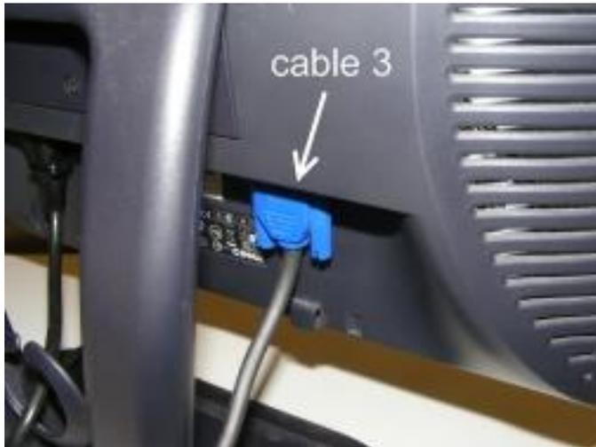
3. Plug one end of **cabl e 3** into the appropriate port on the monitor.
