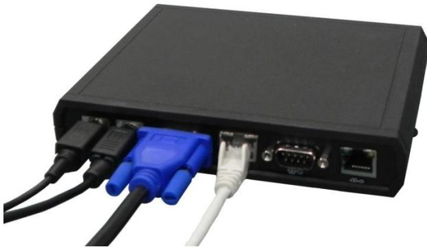
4. Plug **end 2** of  **cable 2**, the **bump bar**, and the remaining end of  **cable 3** into the **Logic Net LS9000**.
