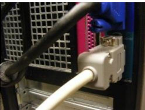
2. Plug the serial cable connected to the scale into the port.
