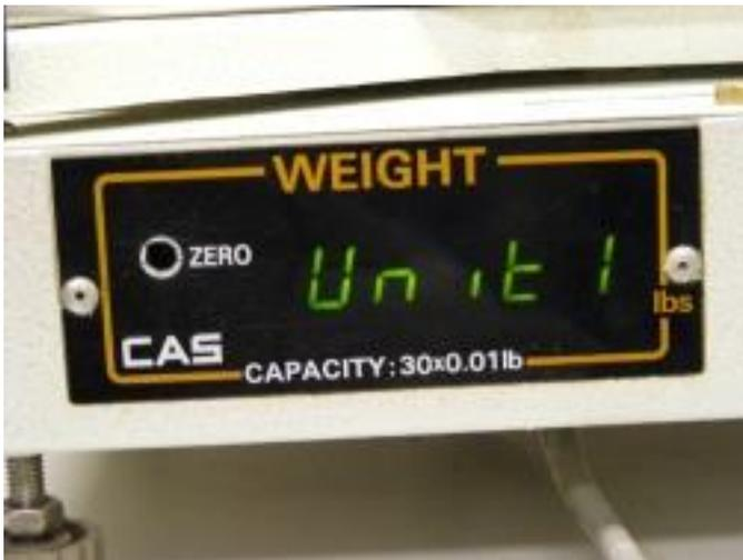
8. You should see “Unit” and a number on the display. This number determines what unit the scale will use:
