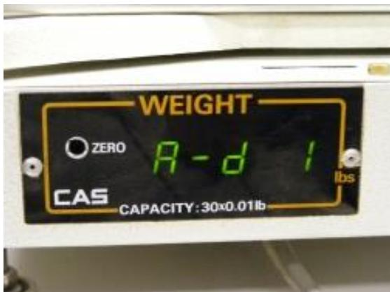
4. The weight display will flash "CAL" three times. After this occurs, release **SW3**. You should see "A-d 1" on the display.
