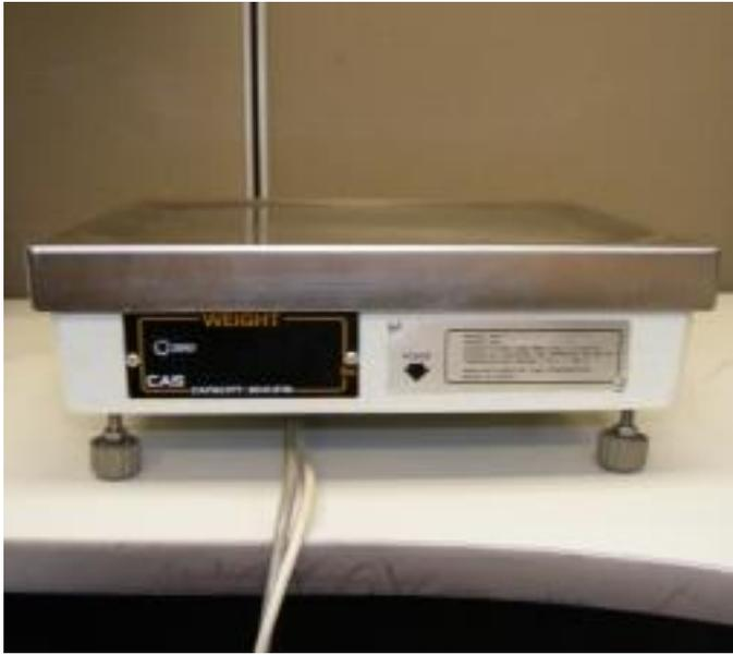
12. Turn the scale off and place the platter properly on the platform.
