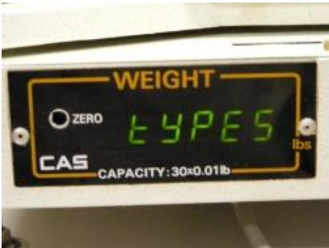
10. You should see “tYPE” and a number on the display. This number determines the scale’s interface type. Press **SW4** until the number is **5**.
